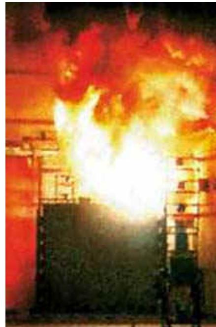
Medium-voltage switchgear being tested under short-circuit conditions. This explosion was created under laboratory conditions to test equipment during arc faults. (courtesy Cutler-Hammer division of Eaton Corporation)
